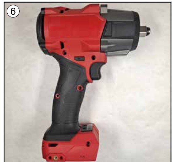
Install right handle halve (cover) over left handle halve (support). Check for the proper functionality of switch and shuttle. Secure handle halves together with seven screws.
