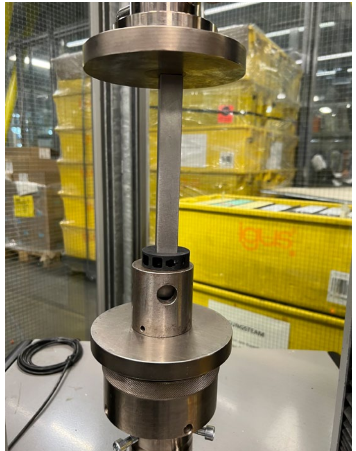
Split fixing collar in the test
