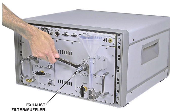
Figure 5. Installing the exhaust filter/muffler
