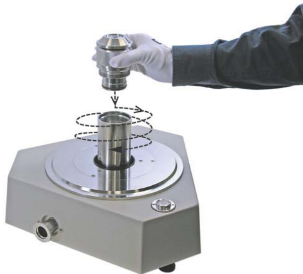
Figure 13. Piston-cylinder module installation
