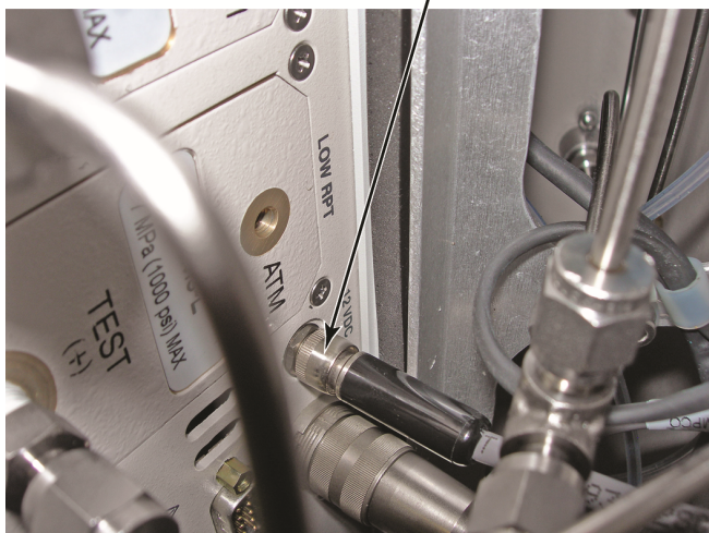
Figure 5: Internal view detail: knurled nut to RPM4
