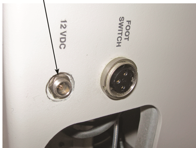
Figure 3: Rear view detail: power supply connection
