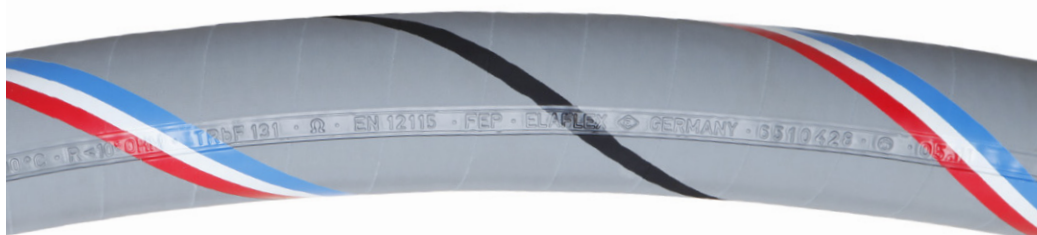
Example ELAFILON PLUS FEP - max. 10^6 Ohm resistance between hose end fittings - not conductive through the hose wall. According EN 12115 so far classified as M hose, according EN 12115 : 2011 now an \Omega hose.
