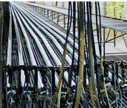
hoses during vulcanizing process
