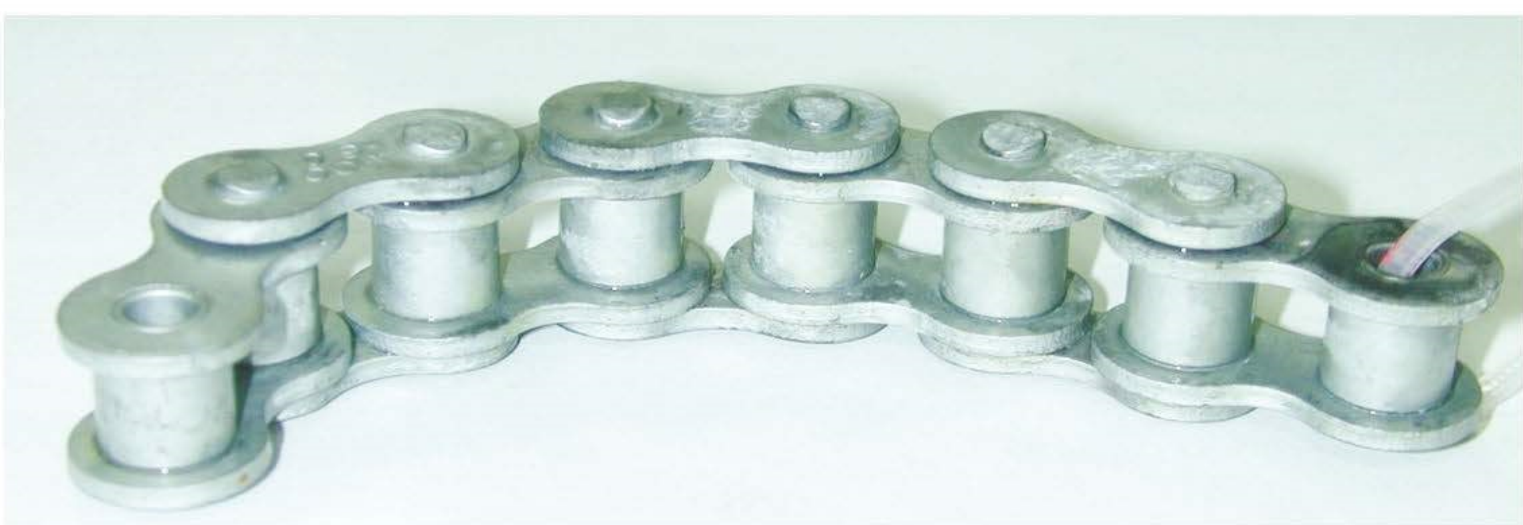
Photo of CR-Chain after Salt Spray Test of 1200hrs
