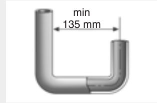
● Minimum clearance of U-shape bends
