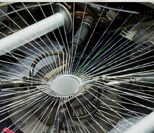
the hollow cone in the weaving loom determines the final diameter
